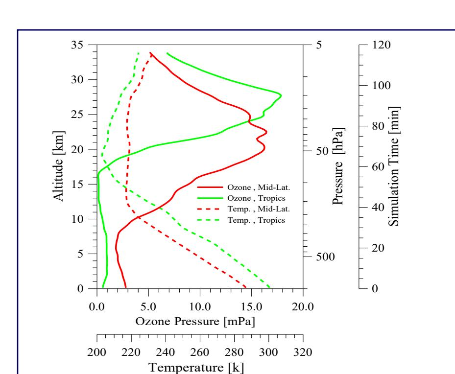
The facility enables control of pressure, temperature and ozone concentration and can simulate quasi realistic flight conditions of ozone soundings to Z=35 km. A dual beam UV-photometer serves as a reference (uncertainty better than ±5 %)
