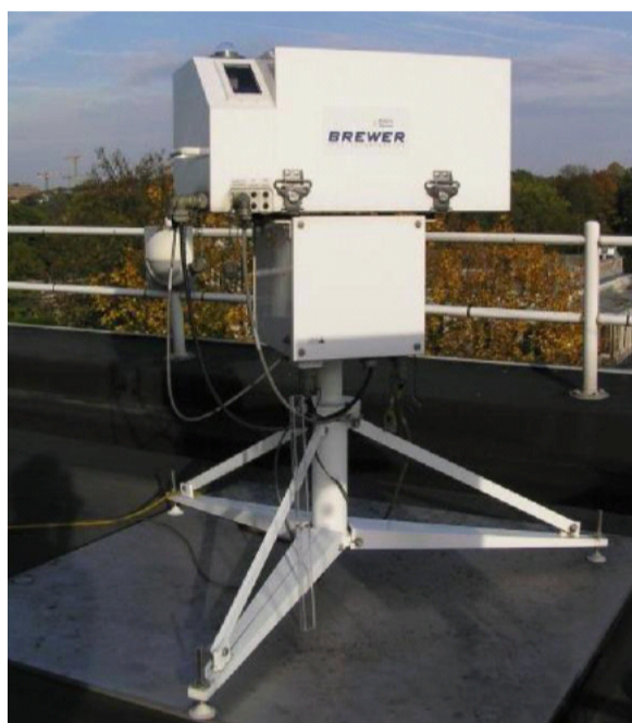
Figure 1. The Brewer spectrophotometer at Uccle.
